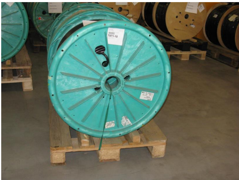
Figure 8: arrangement and marking of cable drums
