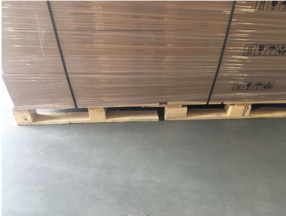
Figure 2: improper overlength pallet
